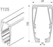
The T125 track, at 125 mm, has the largest span of all Winncare tracks and can be used as a continuous track together with our unique transition gate.
